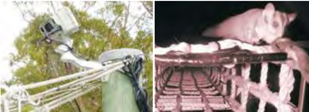
Plate 5.8 Camera to detect species using rope ladder crossing (Faunatech 2020)
